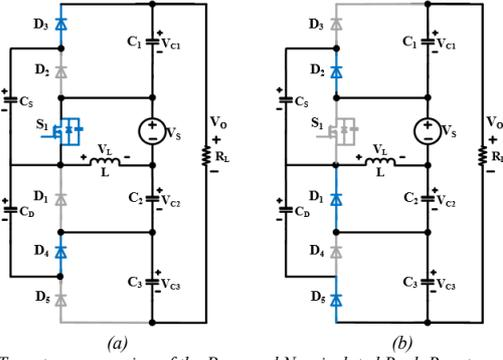
Fig. 3. Two stage expansion of the Proposed Non-isolated Buck-Boost converter
