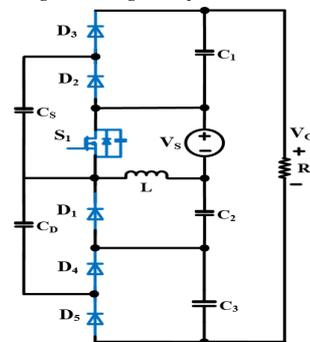
Fig 2. Proposed high-boost converter
