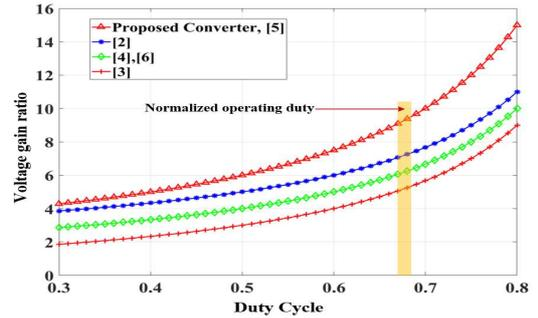
Fig. 5. Voltage gain vs. duty cycle of the high voltage gain converters
