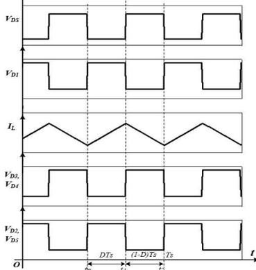
Fig. 4. Key waveforms of proposed converter for CCM operation
