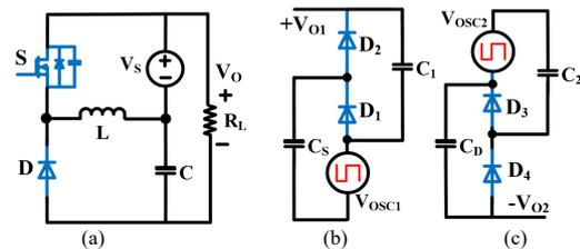
Fig 1. (a) Proposed cascode IBB converter, (b) Positive voltage multiplier. (c) Negative voltage multiplier.
